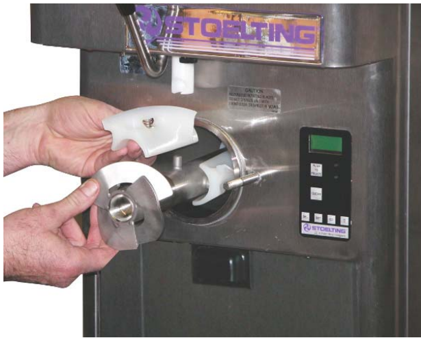
Figure 3-5 Removing Auger Shaft and Flights
