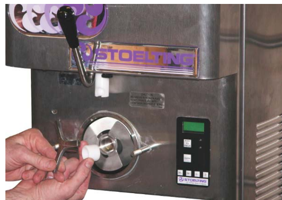
Figure 3-4 Removing Auger Support
