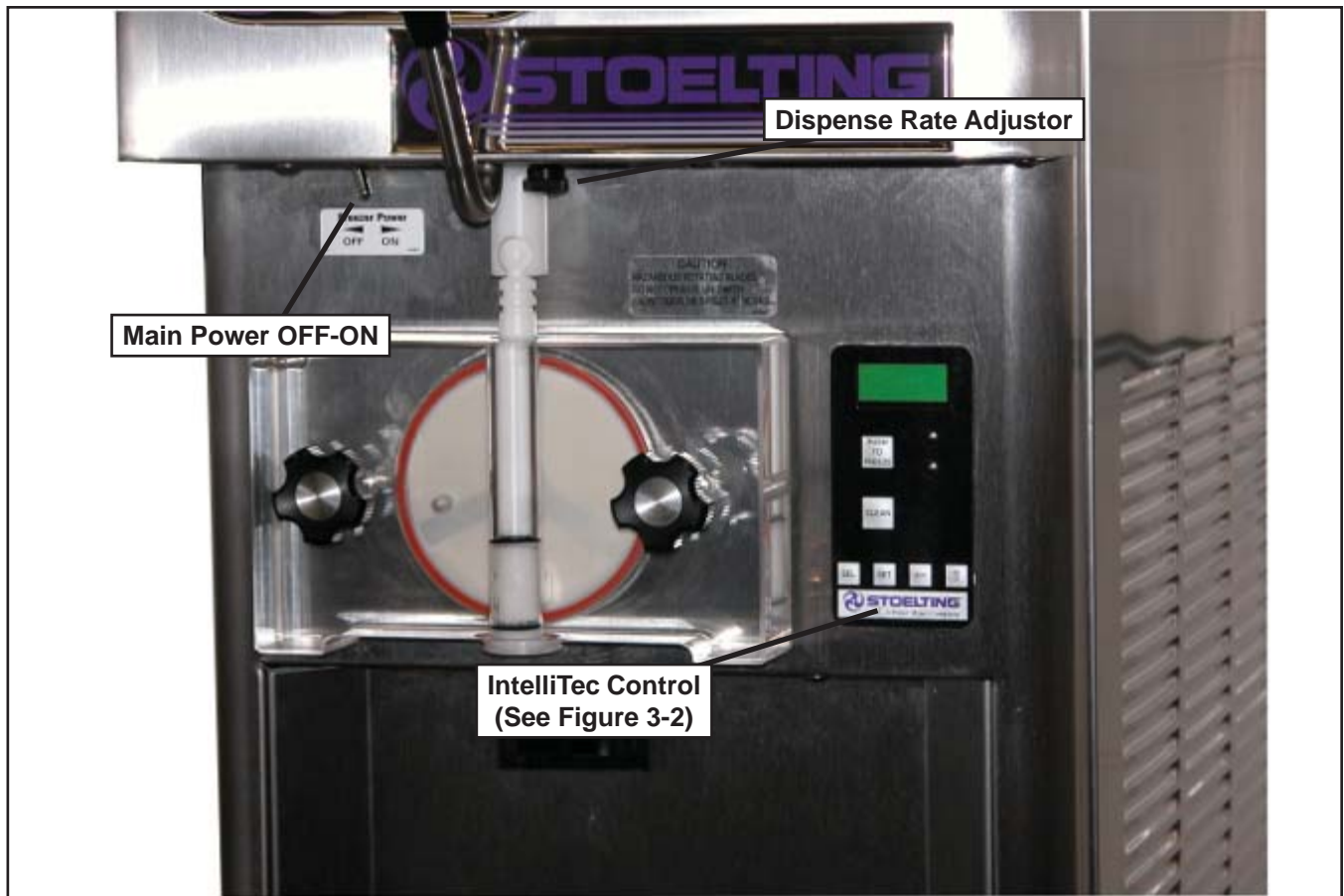
Figure 3-1 E111 & F111 Controls
